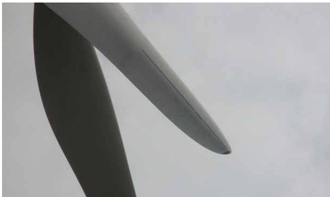
Lightning causes cracks on the blades (Photo: Windplus)
